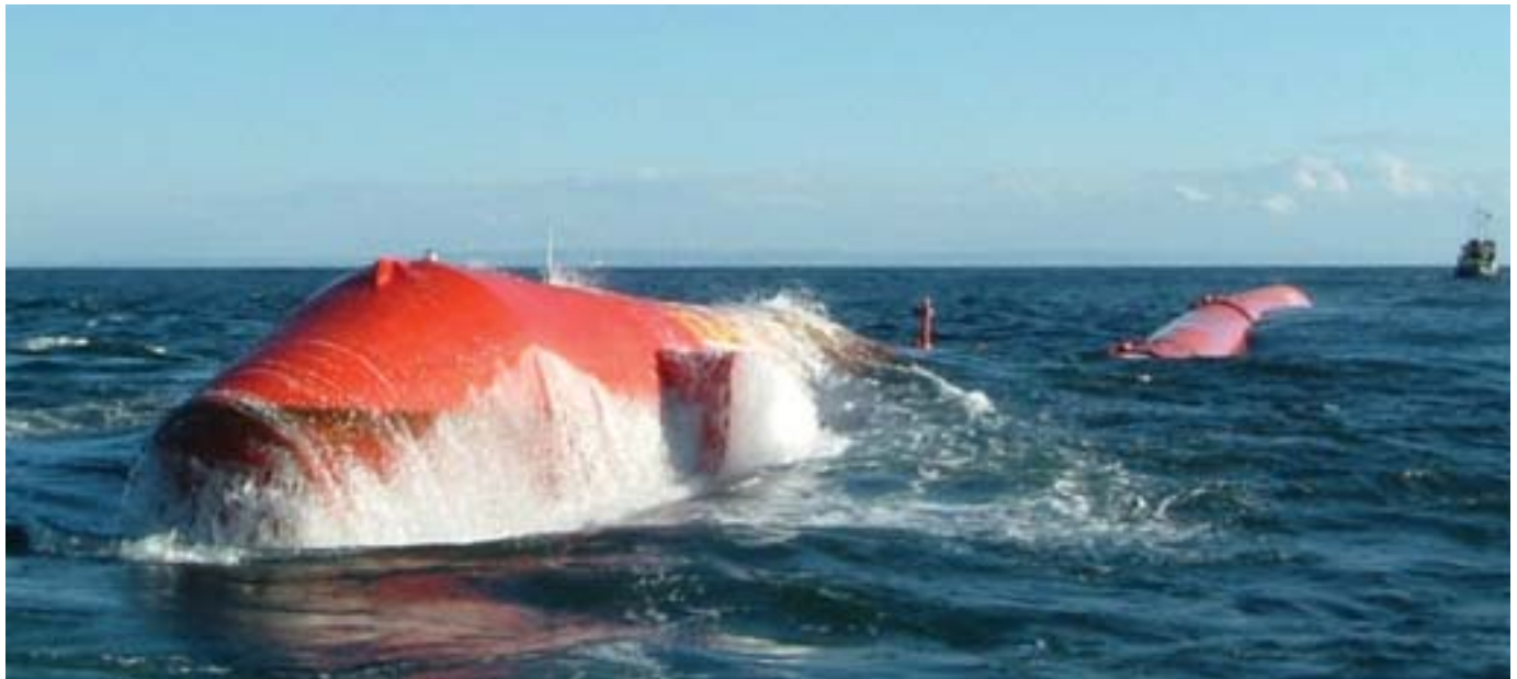
A prototype Pelamis, developed by Ocean Power Delivery Ltd, deployed at the European Marine Energy Centre at Orkney. This site allows developers the opportunity to test and monitor equipment. Such tests provide important information needed when determining future impacts. Photo courtesy of Ocean Power Delivery Ltd.
