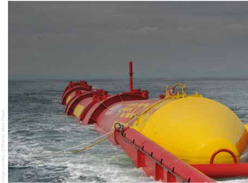
A Pelamis machine ready to convert wave energy into sustainable electricity
